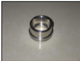
Body ASTM 479/A, 304 Stainless Steel 1.50" diameter x 0.875" thick
